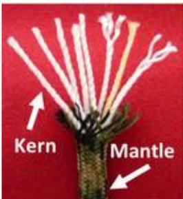
“Kernmantle” type rope or cord is constructed with a removable interior core, called the “kern.” The kern is also sometimes referred to as the “guts” of the cord. The “kern” is protected by a woven outer sheath, called the “mantle.”
