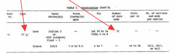
1/ The core yarn shall be constructed by plying five yarns of 210 denier, resulting in a 1050 denier yarn, for the initial spin, or by using 1050 denier singles yarn, then plying three of the 1050 yarns (either 5 ply or singles) together, resulting in a final core size of 3150 denier.
