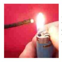
Or, some people prefer to burn the cut ends of the paracord with a lighter, match, "hot knife," or even an inexpensive wood burning tool. This will melt the ends of the nylon together so that they don't unravel.
