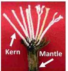
"Kernmantle" type rope or cord is constructed with a removable <u>interior</u> core, called the "kern." The kern is also sometimes referred to as the "guts" of the cord. The "kern" is protected by a woven outer sheath, called the "mantle."
